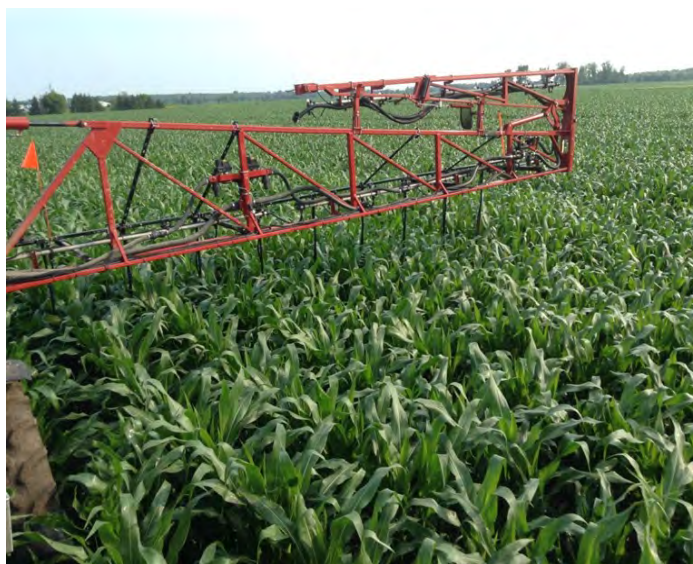
Figure 2— Y Drop in field application- Vernon Valley Farms Ltd. July 2015
