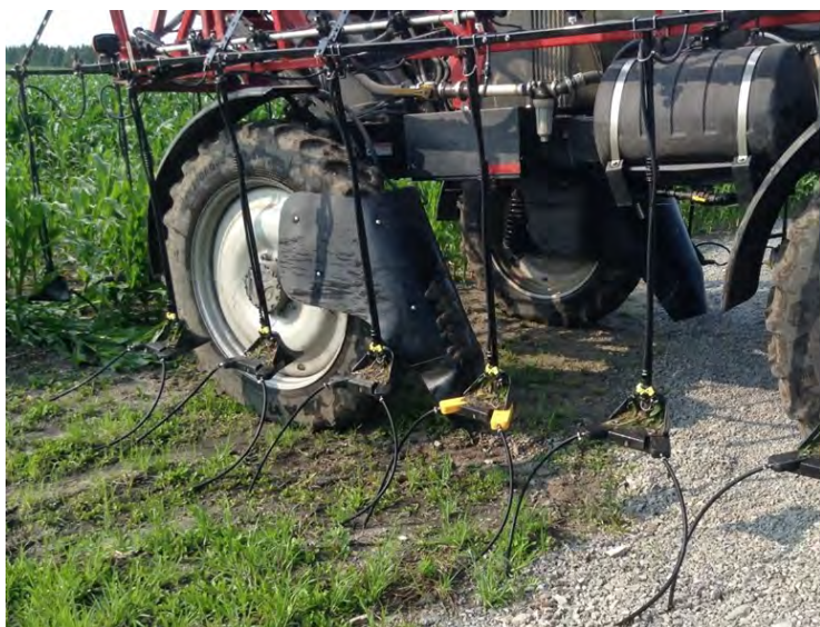
Figure 1- Y Drop row unit applicators - Vernon Valley Farms Ltd. July 2015
